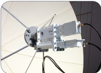
ZF300 mounted on a parabolic antenna feed
